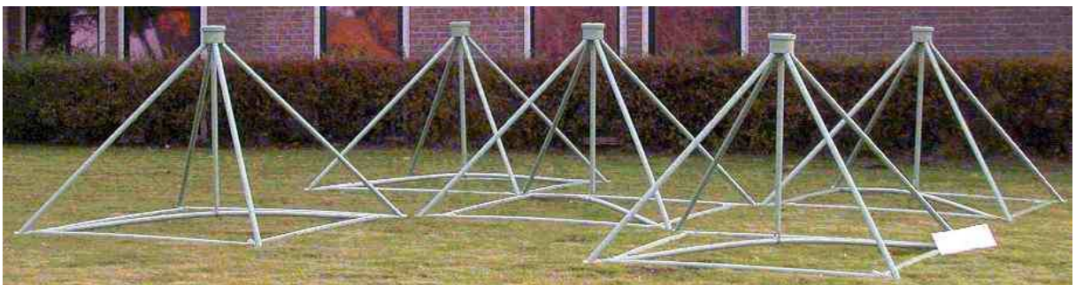
Figure 1: Prototype low-band (30–80 MHz) LOFAR antennae of the type that have been deployed at the LOFAR Initial Test Station (ITS) and Core Station One (CS1). Eventually up to 5000 such antennae will be distributed across the Netherlands, in 36-50 stations each containing 96 antennae (plus 48 high-band tiles).
