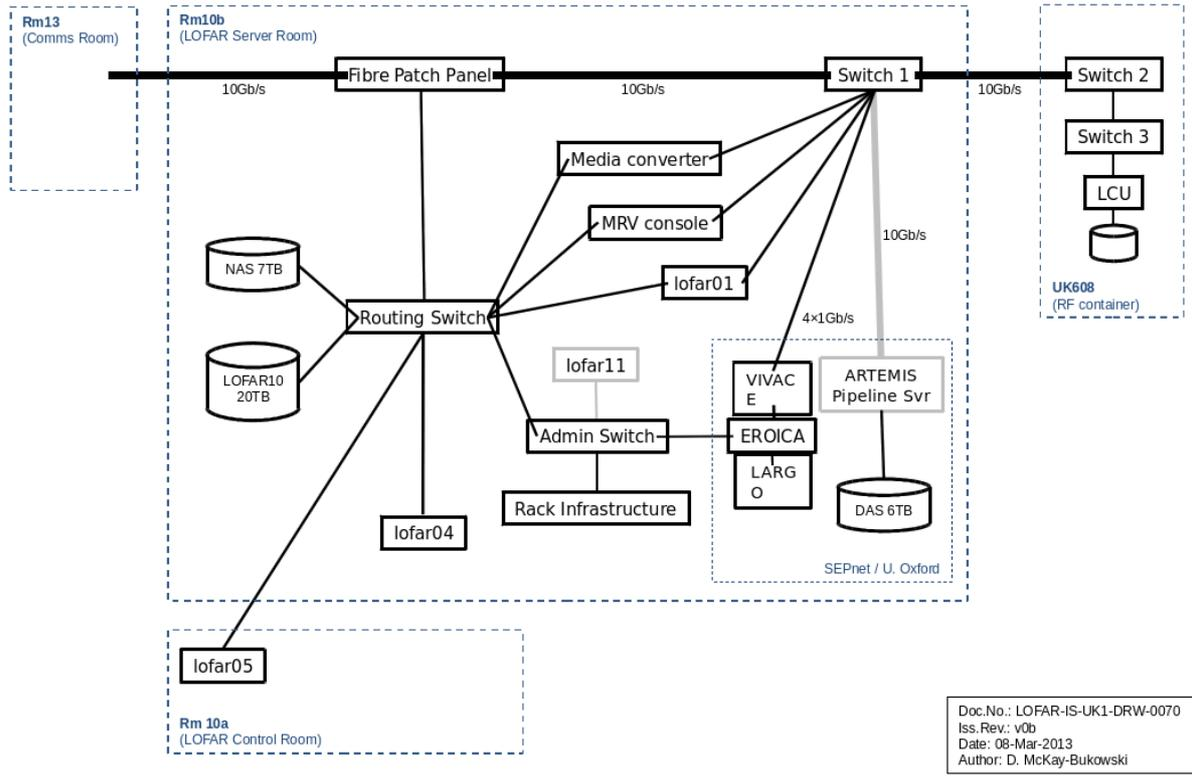
Figure 1: This figure shows the computing layout for the UK608 network. Access to the station from the outside world is through LOFAR01, from which the other units may be accessed. Statistics are recorded directly on the LCU, and later moved to to NAS\_DATA for storage. Data requiring further processing via ARTEMIS flows from the station LCU to the processing units VIVACE or LARGO, and then finally to either the storage units NAS or OFFLINE\_NS.
